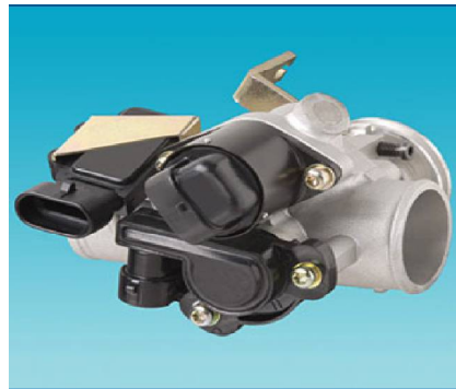
Fig No 01 Engine Throttle butterfly valve
